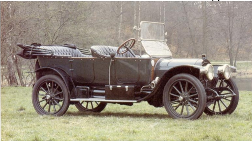
Brass-age car with nickel trim all over - the owner does not have to polish to keep the stuff shining. I've been told that nickeling was quite fashionable in 1913. On the near-side what the Danes call a 'snijdedor' (cheating door) - there is no door!
