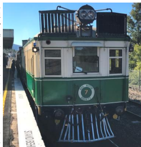
Cow catcher & roof radiators.
