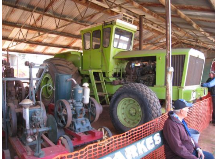
'Orphan Annie', built in 1979, has a 350 HP Cummins engine.
