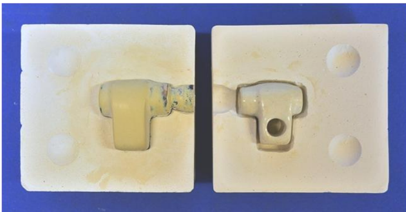
LHS - Timber pattern placed in mould. RHS - Fired porcelain insulator in mould, now notice the amount of shrinkage that has occurred.
