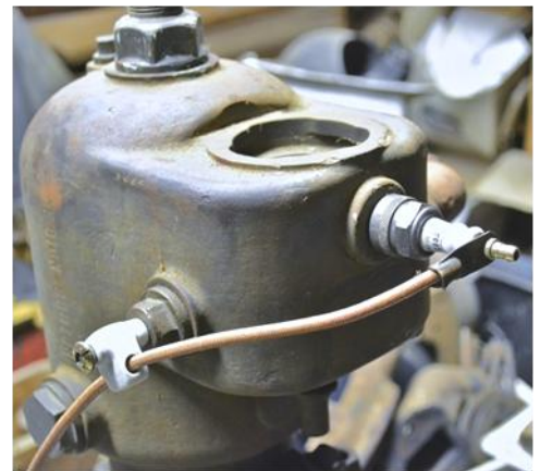
Showing location of porcelain insulator when fitted to cylinder block
