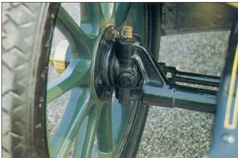
No front-wheel brakes. The front axle design is simple but effective
