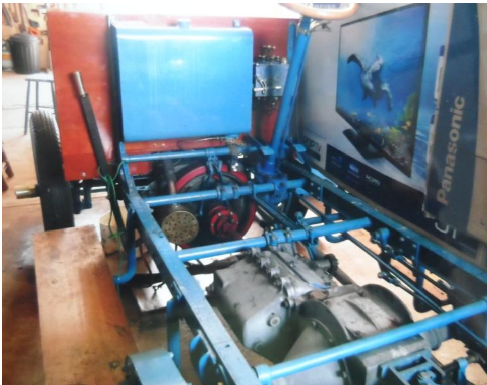
Starting on the bodywork. Note the gearbox/differential. Cardboard for profile on side.
