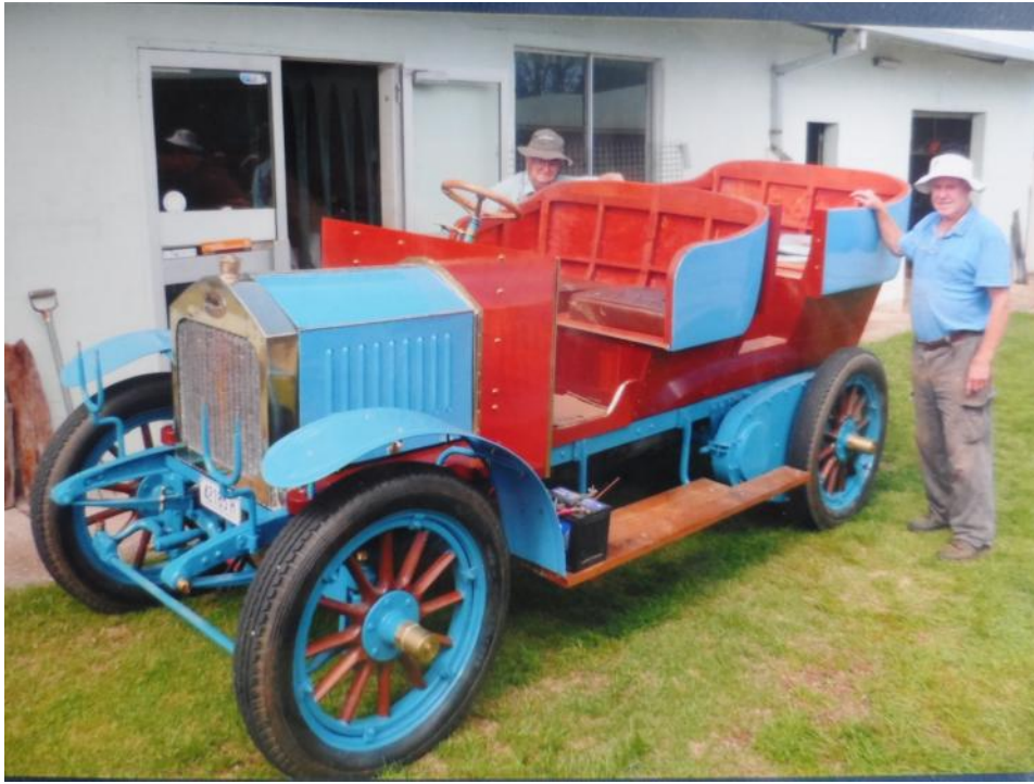
Metal parts painted and woodwork ready for upholstery
