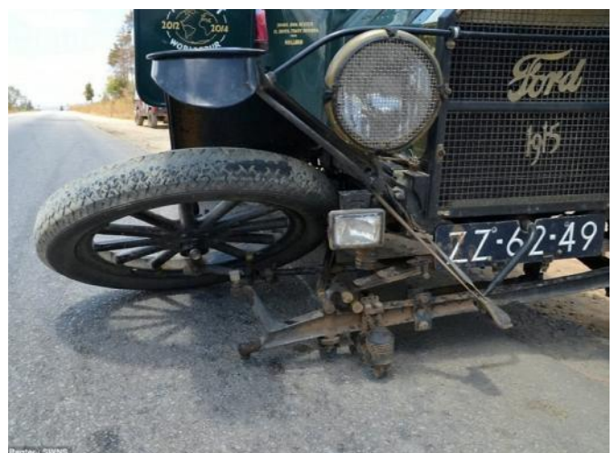
Another mishap - broken king pin.
