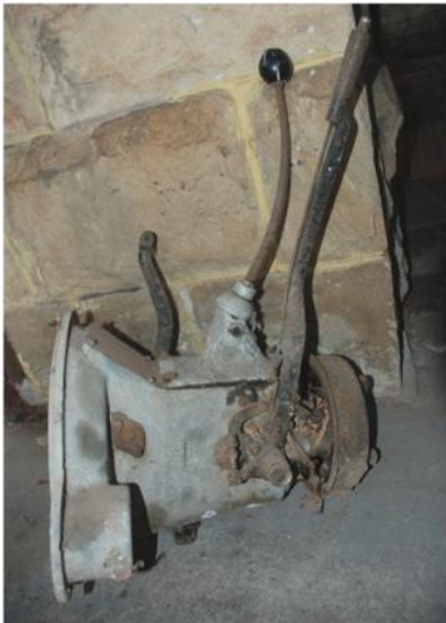
The mystery gearbox has been identified as a 1922 Crossley gearbox.
